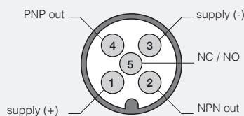
CX0RP/\*\*\_\*\*-\*\* receiver with PNP output and Teach-In function
