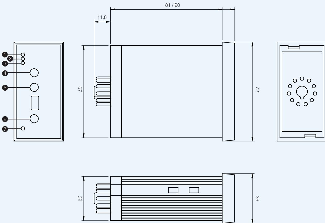
Holes dimensions for mounting on panel: 68x33 mm.
