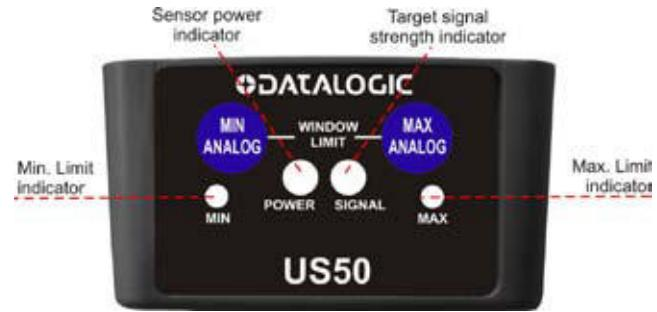
**Signal LED (Red)** – indicates the strength and condition of the sensor's incoming signal.
