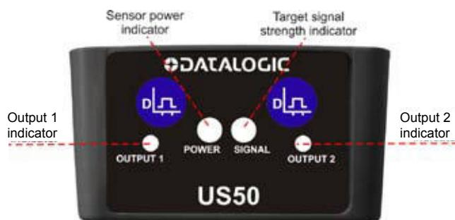
**Signal LED (Red)** – indicates the strength and condition of the sensor's incoming signal.
