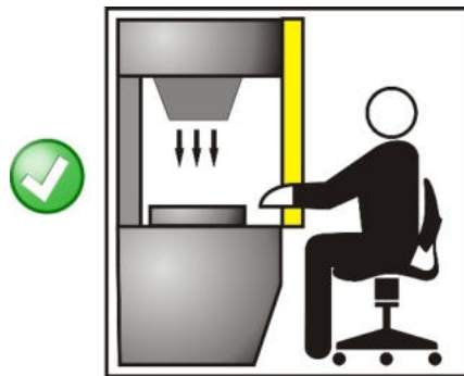
Fig 10 - Correct light curtain positioning
