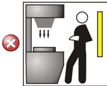
Figure 3 - Wrong light curtain positioning
