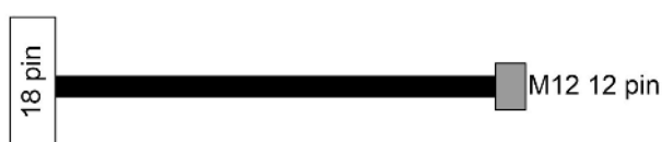
Figure 3 - Pigtail cable Blanking configuration for receiver (CS-G1-70-B-002)
