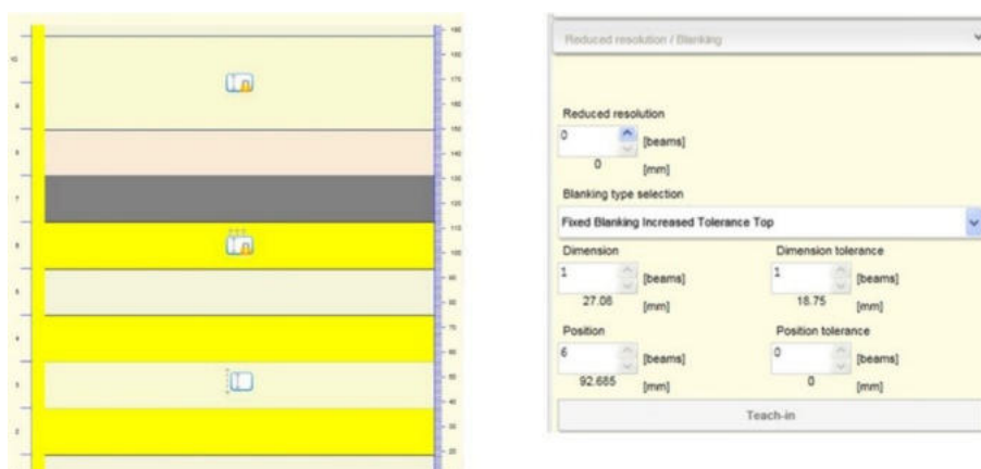
Figure 59 - Fixed Blanking with increase tolerance
