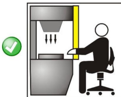
Figure 2 - Correct light curtain positioning
