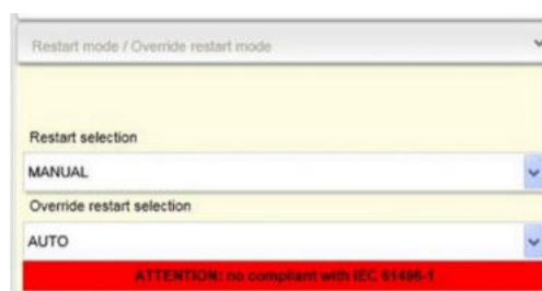
Figure 42 - ACM Configuration: Auto Override Restart Selection
