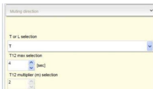
Figure 25 - ACM Configuration: Muting direction
