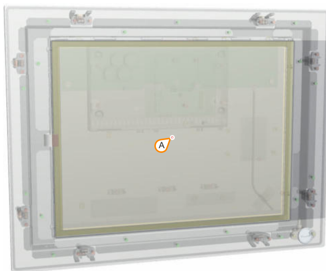
Figure 3: Automation Panel 1000 - Temperature sensor position
