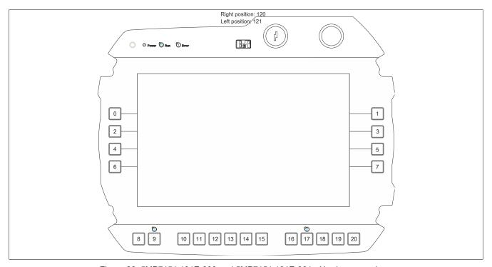
Figure 28: 5MP7151.101E-000 and 5MP7151.101E-001 - Hardware numbers
