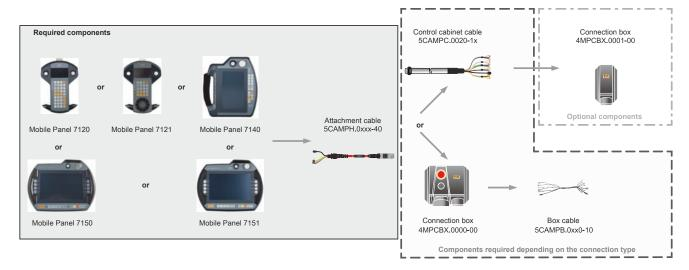
A attachment cable type with different lengths is available for selection for the Mobile Panel 7100 (5CAMPH.xxxx-40). This cable is required regardless of the selected connection type. It is possible to choose between the following connection types:
