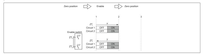
Figure 3: Contact travel diagram for normal actuation
