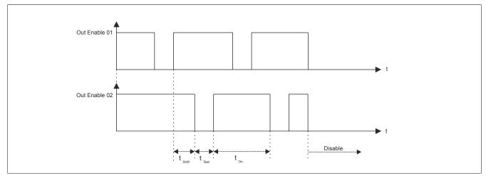
Figure 5: Enabling electronics - Testing for short circuits and cross faults
