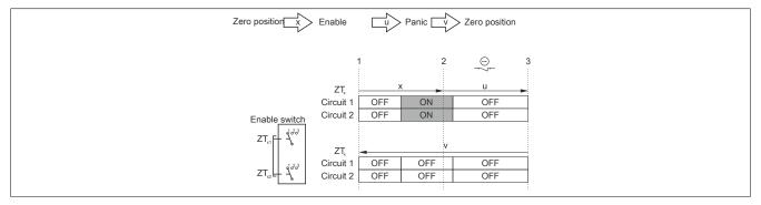
Figure 4: Contact travel diagram for panic actuation
