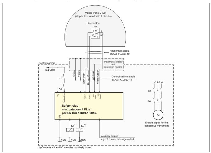
Figure 23: Connection example for stop button for MP7100
