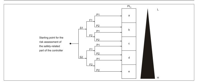
Figure 29: Risk graph for determining the PLr for each safety function
