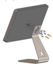
4. The panel can be rotated 90° by loosening the screws.
