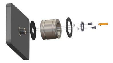
6. Connect the cable to the panel and secure it before the panel (including the preinstalled flange adapter) is screwed in place.
