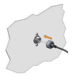
6. Tighten the cable gland (Torque: 3.0 Nm).
