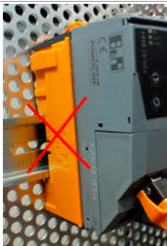
Figure 3: X20 system - Removing the end cover plates
