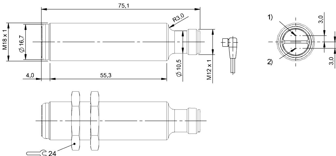
1) Optical axis receiver, 2) Optical axis emitter
