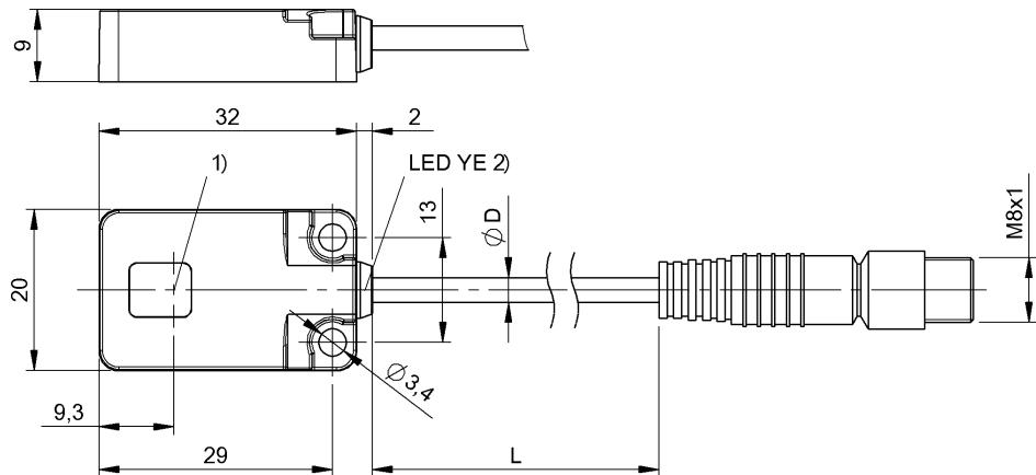
1) Optical axis receiver, 2) Output function
