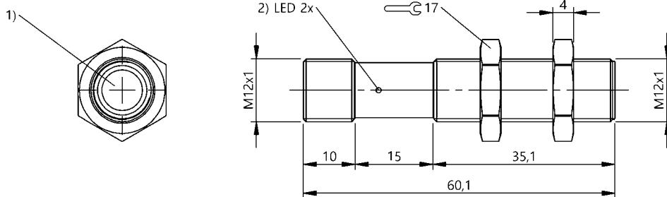
1) Ultrasonic transducer axis, 2) Function indicator
