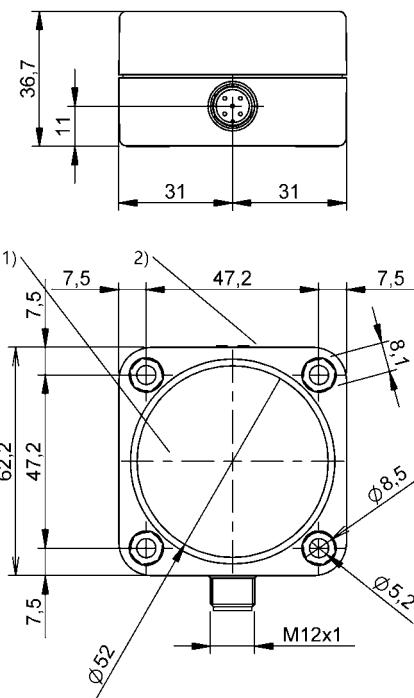
1) Ultrasonic transducer, 2) Display and control panel
