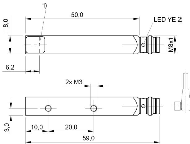
1) Optical axis receiver, 2) Output function
