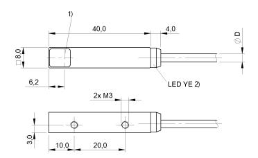
1) Optical axis receiver, 2) Output function
