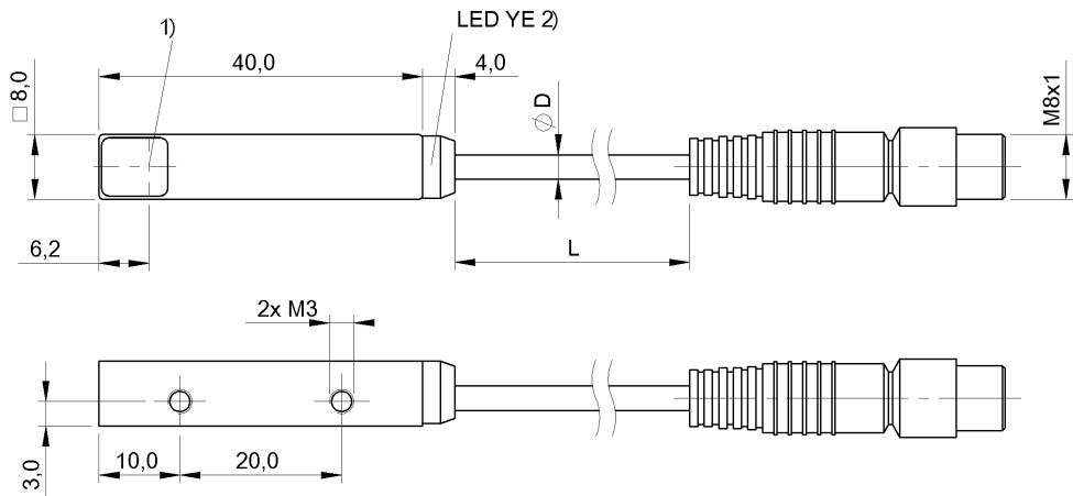
1) Optical axis receiver, 2) Output function
