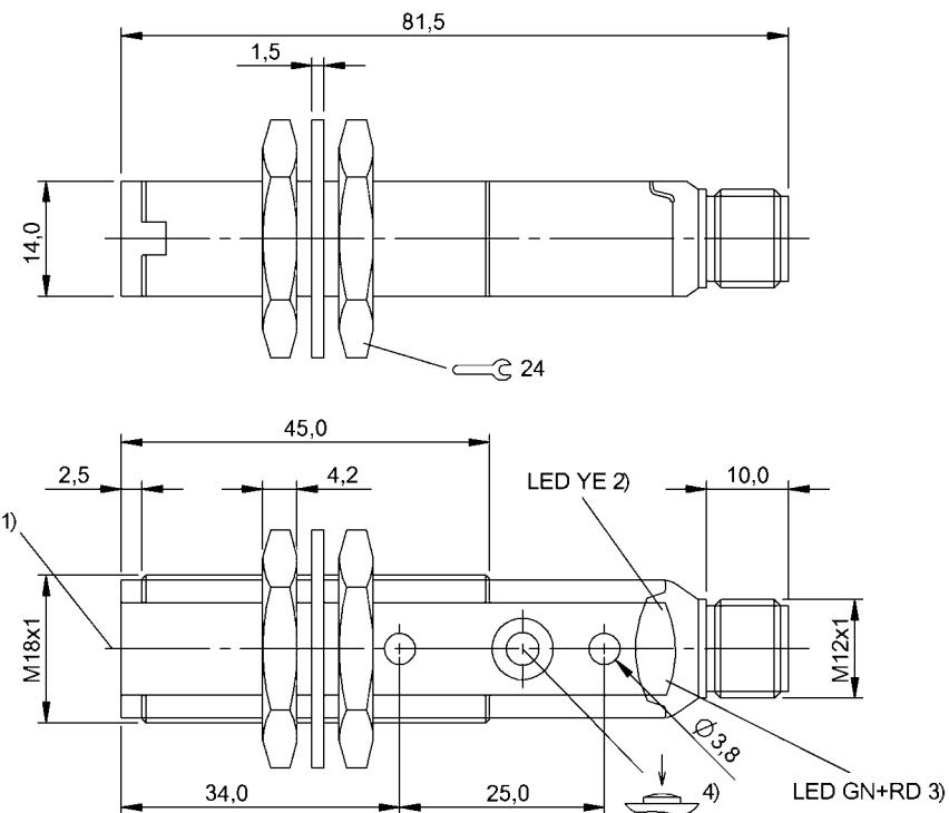
1) Optical axis, 2) Output function, 3) stability/error, 4) Sn
