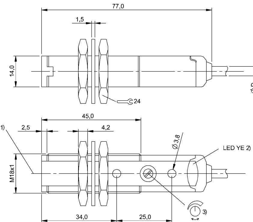
1) Optical axis, 2) Output function, 3) Sn
