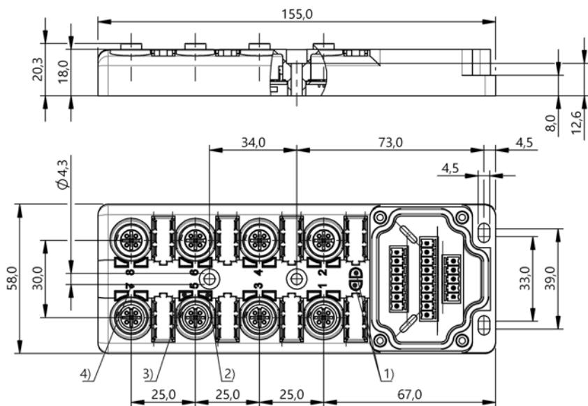
1) Power ind. green potential, 2) LED ye for S2 on PIN 2, 3) LED ye for S1 on PIN 4, 4) Slot numbering
