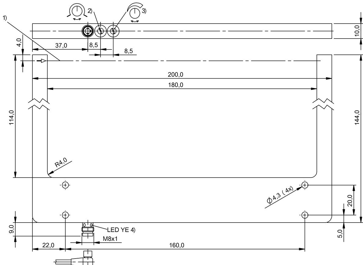
1) Optical axis, 2) Sensitivity, 3) Light-on/dark-on, 4) Output function
