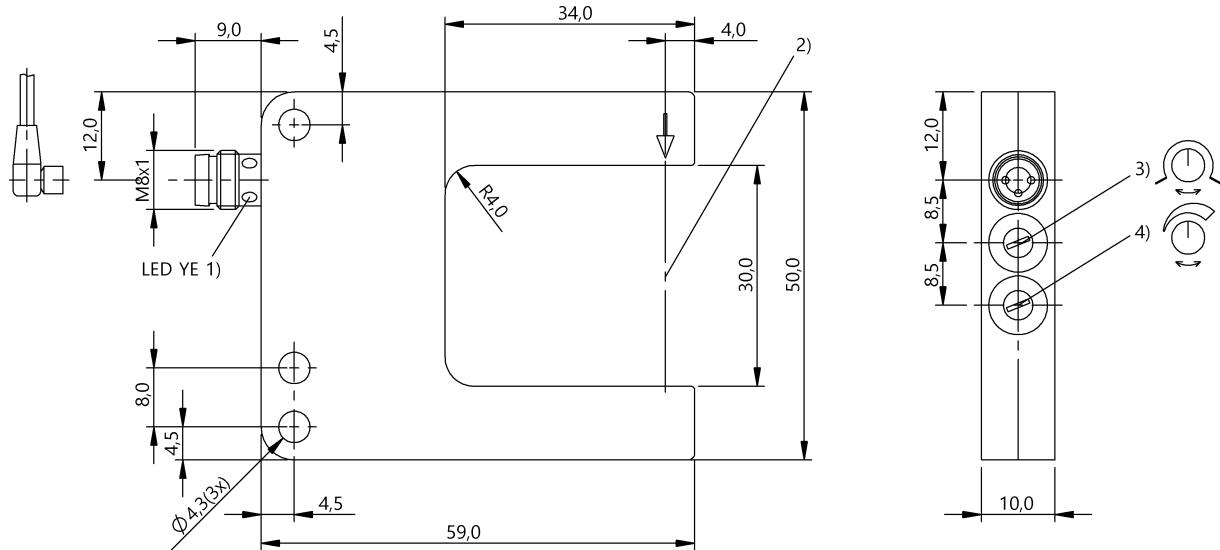
1) Output function, 2) Optical axis, 3) Light-on/dark-on, 4) Sensitivity
