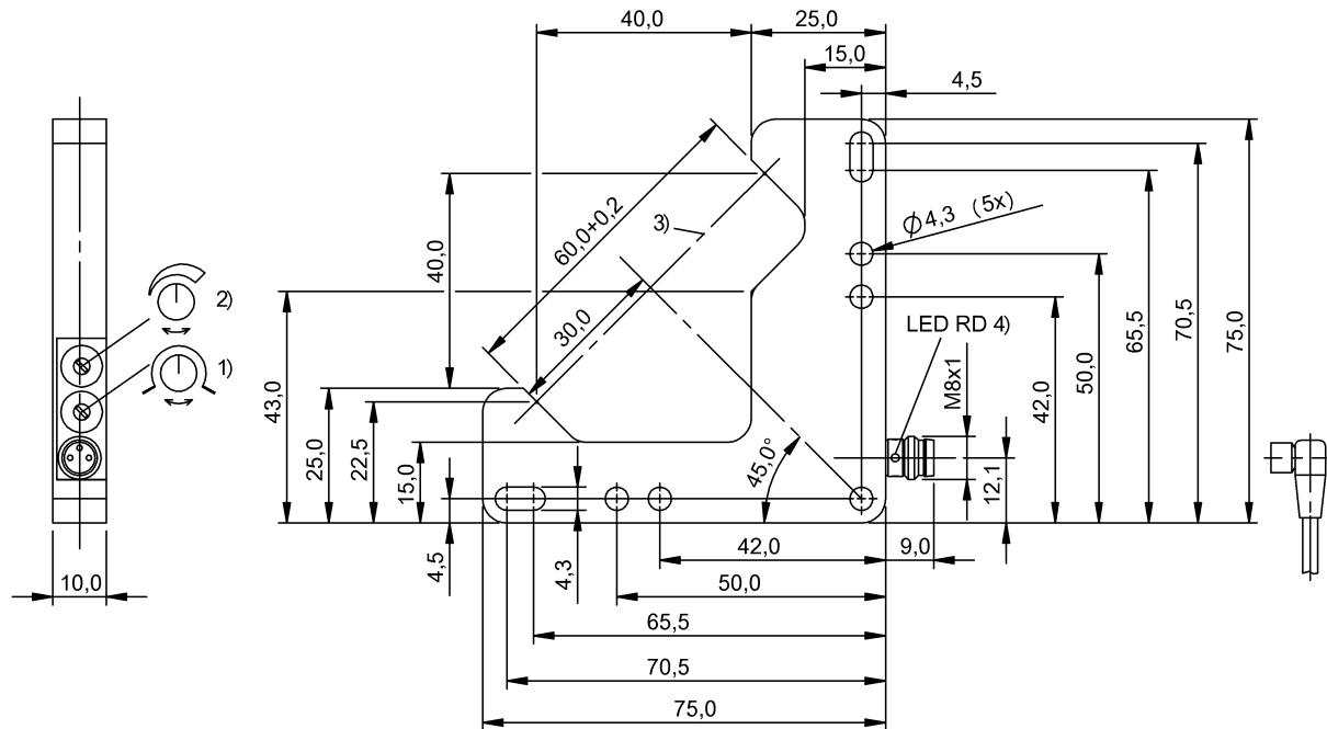
1) Light-on/dark-on, 2) Sensitivity, 3) Optical axis, 4) Output function
