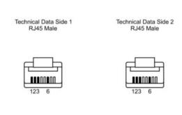
Color Code 1 = WH/OR 3 = WH/GN 2 = OR 6 = GN Shield = RJ45 Sleeve Color Code 1 = WH/OR 3 = WH/GN 2 = OR 6 = GN Shield = RJ45 Sleeve
