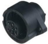
Circular Receptacle Power Connector (CA Series): Female, front mount with flange, 7-pin(6+PE), 230 V AC/DC, 10 A
