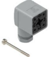
GDM DIN Valve Connector, Form A, 18mm, 2+Ground, M16x1, Grey Housing, with circuit (Bridge Rectifier and Varistor), 250 V | 1 A, Steel Center Screw, Bulk Packaging
