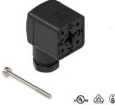
GDM Standard DIN Standard Field Attachable Connector: Form A, 3-pin (2+1PE; PE across cable outlet), UL 2238, black housing, screw type, M16 with strain relief; without circuitry, 230 V AC/DC, 10 A
