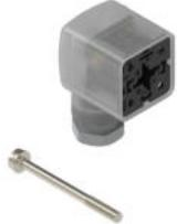
GDM Standard- 175301-803 (DIN 43650), Form A, 18mm, 2 Pole+Ground (Protective Earth), Translucent Housing, M16 Grey Gland Nut, PCBA with Yellow LED, and Varistor, 24V | 10 A, Steel Center Screw, Bulk Packaging
