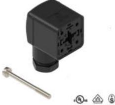
GDM Standard DIN Standard Field Attachable Connector: Form A, 4-pin (3+1PE; PE across cable outlet), black housing, screw type, PG11; without circuitry, 230 V AC/DC, 16 A
