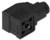
Heavy Duty: DIN Valve Connector, Form A, Field Attachable, 3+Ground, PG 13.5, Black Housing, without circuitry, 230 V DC / 400 V AC AC/DC
