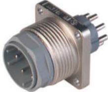
N11R, M26 x 1.5 thread, Field Attachable, Male, Surface Mount with Flange, Metal housing, AC 25 V / DC 50 V, 5 A
