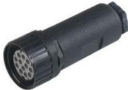
N11R, M26 x 1.5 thread, Field Attachable, Female, Straight, Black housing, 60 V, 5 A, PG 16 w/ strain relief and clamping cage
