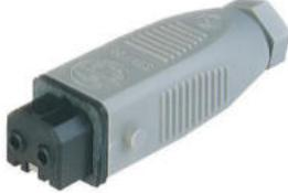
Rectangular Field Attachable Power Connector (ST Series): Female, straight with strain relief, 2-pin+PE, grey housing, 230 V AC/DC, 16 A AC/6 A DC
