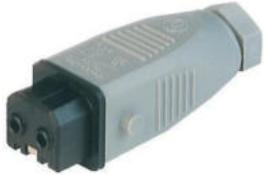
Rectangular Field Attachable Power Connector (ST Series): Female, straight, 2-pin+PE, grey housing, 230 V AC/DC, 16 A AC/6 A DC
