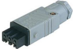
Rectangular Field Attachable Power Connector (ST Series): Female, straight with strain relief, 3-pin+PE, grey housing, 400 V AC/230 V DC, 16 A AC/10 A DC
