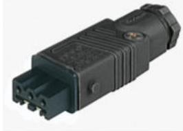
Rectangular Field Attachable Power Connector (ST Series): Female, straight with strain relief, 3-pin+PE, black housing, 400 V AC/230 V DC, 16 A AC/10 A DC
