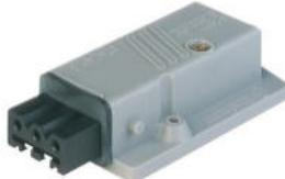
Rectangular Receptacle Power Connector (ST Series): Female, panel mount, 3-pin+PE, grey housing, 400 V AC / 230 V DC, 16 A AC/10 A DC
