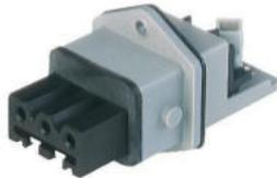
Rectangular Receptacle Power Connector (ST Series): Female, front mount with flange, 3-pin+PE, grey housing, 400 V AC / 230 V DC, 16 A AC/10 A DC
