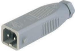
Rectangular Field Attachable Power Connector (ST Series): Male, straight with strain relief and coding slot , 2-pin+PE, grey housing, 230 V AC/DC, 16 A AC/6 A DC
