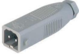
Rectangular Field Attachable Power Connector (ST Series): Male, straight with strain relief, 2-pin+PE, grey housing, 230 V AC/DC, 16 A AC/6 A DC
