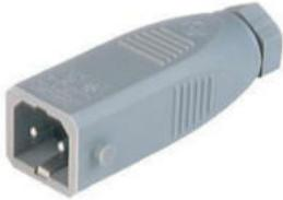
Rectangular Field Attachable Power Connector (ST Series): Male, straight, 2-pin+PE, grey housing, 230 V AC/DC, 16 A AC/6 A DC
