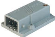
Rectangular Receptacle Power Connector (ST Series): Male, panel mount, 3-pin+PE, grey housing, 400 V AC / 230 V DC, 16 A AC/10 A DC
