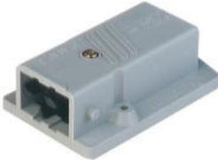
Rectangular Receptacle Power Connector (ST Series): Male, panel mount, 5-pin+PE, grey housing, 400 V AC / 230 V DC, 10 A AC/6 A DC
