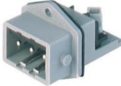
Rectangular Receptacle Power Connector (ST Series): Male, front mount with flange, 3-pin+PE, grey housing, 400 V AC / 230 V DC, 16 A AC/10 A DC
