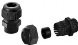
Metric cable glands MBF, polyamide, black, IP 68 (5 bar, 30 min)
