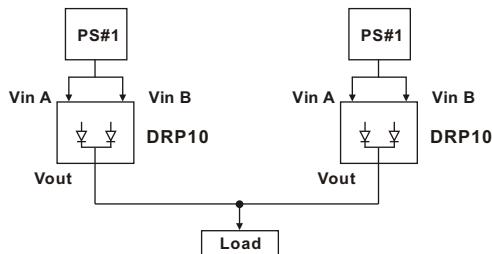
3.) 1+N Redundancy : Using 1 more PS as the redundant units to increase the reliability.
