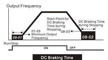
NOTE: 1. DC Braking during Start-up is used for loads that may move before the AC drive starts, such as fans and pumps. Under such circumstances, DC Braking can be executed to hold the load in position before applying a forward motion.
