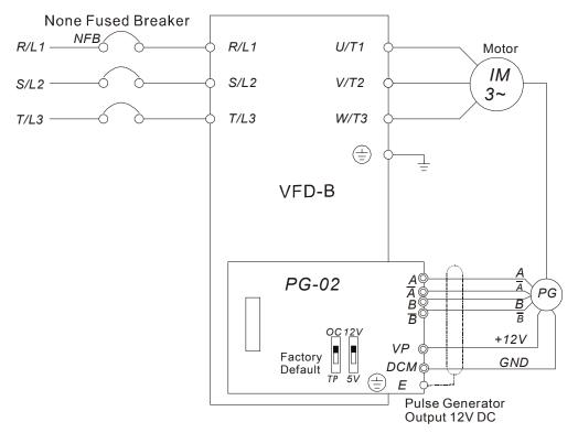
PG-02 and Pulse Generator Connections
