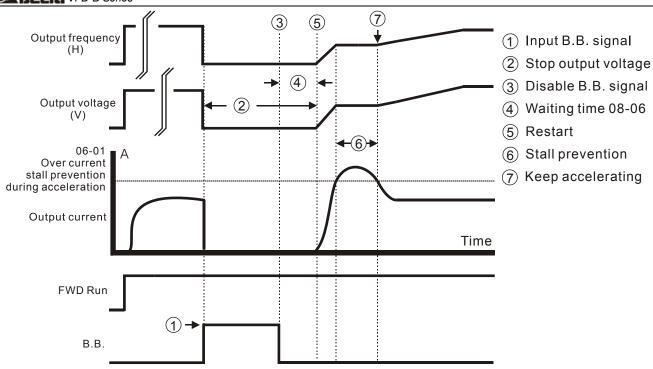
Fig 3: B.B. Speed Search with Minimum Output Frequency Upward Timing Chart (Start-up Current Attains Stall Current Level)
