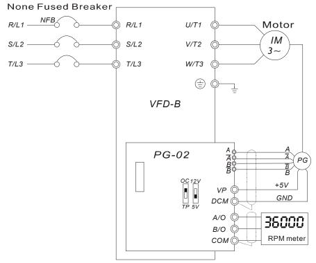
PG-02 and Pulse Generator Connections
