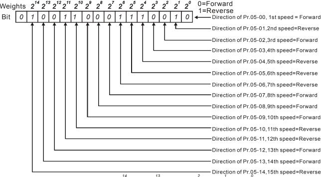
The setting value = bit14x2<sup>14</sup>+bit13x2<sup>13</sup>+....+bit2x2<sup>2</sup>+bit1x2<sup>1</sup>+bit0x2<sup>0</sup> = 1x2<sup>14</sup>+1x2<sup>17</sup>+1x2<sup>10</sup>+1x2<sup>6</sup>+1x2<sup>5</sup>+1x2<sup>4</sup>+1x2<sup>1</sup> =16384+2048+1024+64+32+16+2 =19570 Setting 05-16=19570
