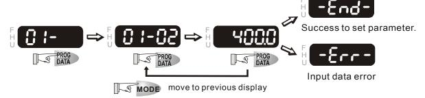
NOTE :In the parameter setting mode, you can press MODE to return the selecting mode.
