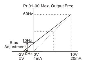
Factory Settings Pr. 01-00 = 60Hz--Max. output Freq. Pr. 04-11 = 20.0%-- bias adjustment Pr. 04-12 = 0-- bias polarity Pr. 04-13 = 83.3%-- pot. Freq. gain Pr. 04-14 = 0-- REV motion disable in negative bias Pr. 04-13 =  $\frac{10V}{12V}$  X 100% = 83.3%Negative bias:  $\frac{60-10}{12}$  =  $\frac{10-0}{12}$
