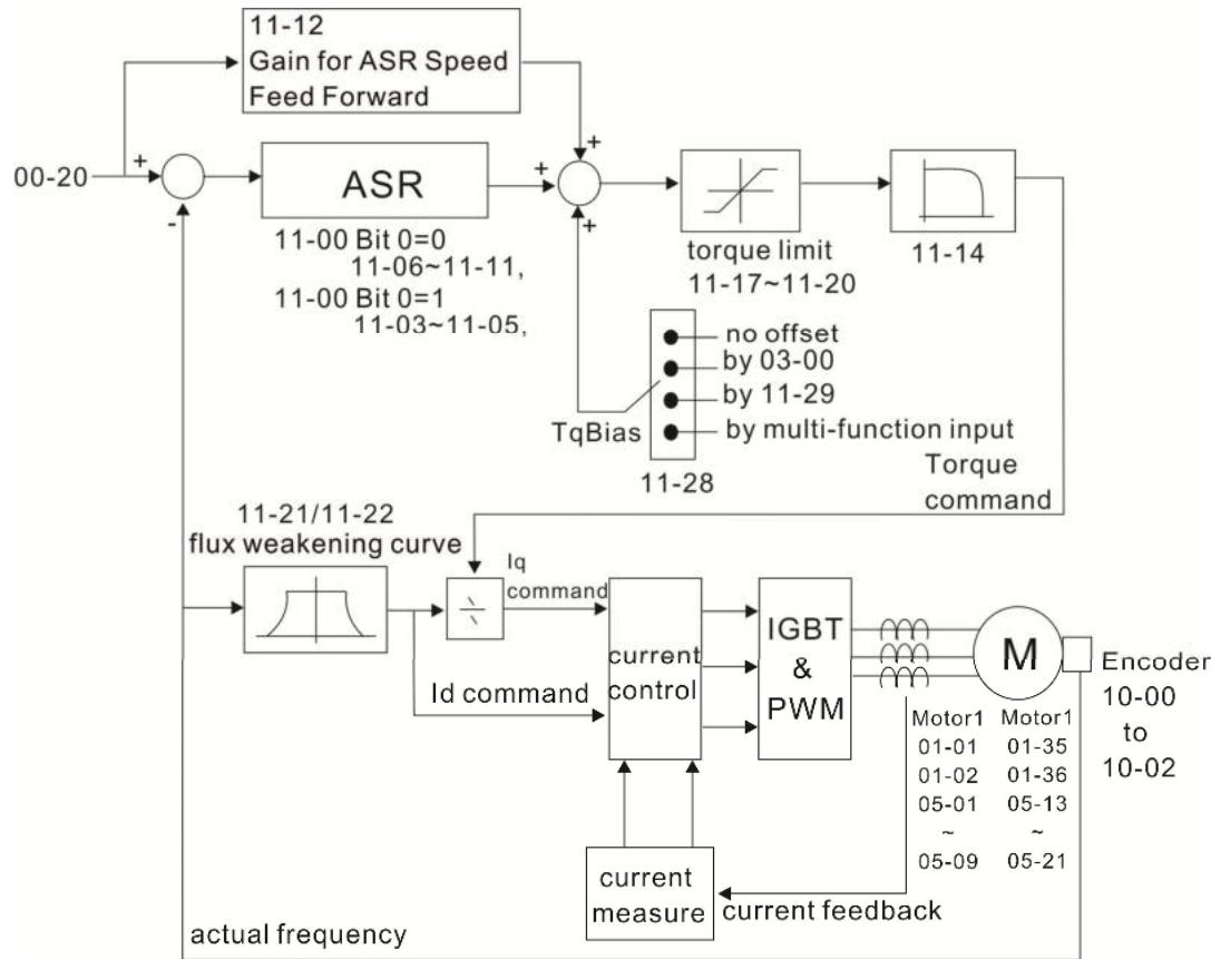
When setting Pr.00-11 to 5, the FOC sensorless (IM) control diagram is shown as follows.
