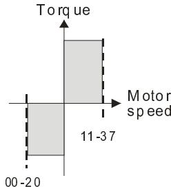
↗ **11-37** Forward Speed Limit (torque mode)
