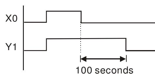
When input X0 is ON, output coil Y1 will be ON at the same time due to the corresponding normally close contact OFF makes timer T10 to be OFF. Output coil Y1 will be OFF after delaying 100 seconds ( $K1000 \times 0.1 \text{ seconds} = 100 \text{ seconds}$ ) once input X0 is OFF and T10 is ON. Please refer to timing chart above.
