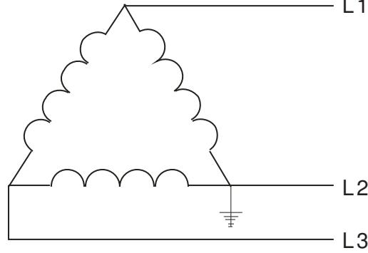
2 Grounding at a midpoint in a polygonal configuration
