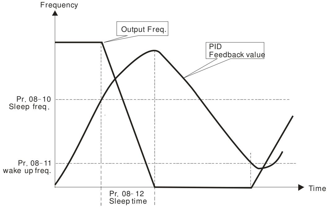
Enable or disable the Sleep and Wakeup functions depends on the setting of Pr08-10. When Pr08-10=0, it means Disable, while Pr08-10 ≠ 0, it means Enable.
