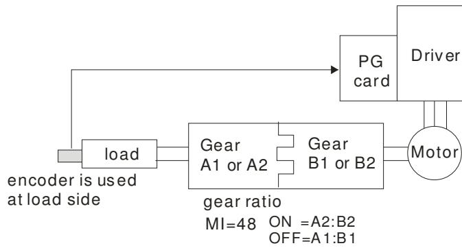
**10 - 08** Treatment for Encoder Feedback Fault
