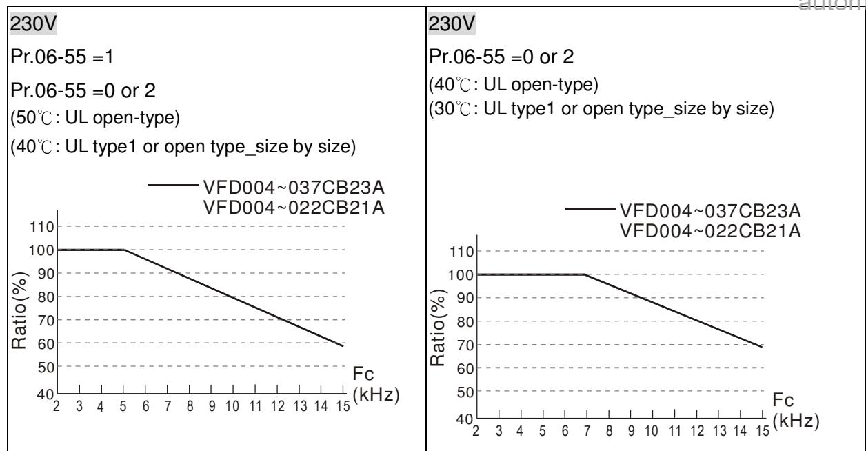
Derating curve diagram in the normal duty (Pr.00-16=0)
