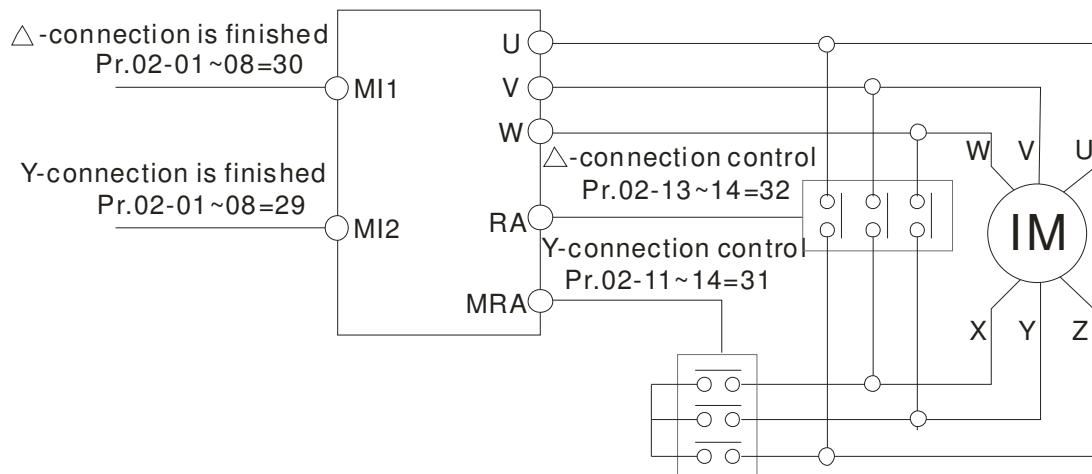
Y-△ connection switch: can be used for wide range motor
