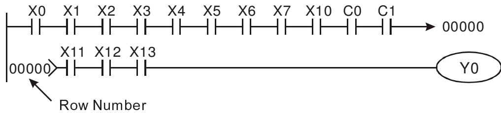
The operation of ladder diagram is to scan from left upper corner to right lower corner. The output handling, including the operation frame of coil and application command, at the most right side in ladder diagram.
