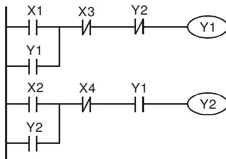
If add normally close contact Y2 into Y1 circuit to be an input for Y1 to do AND function. (as shown in the left side) Y1 is an input of Y2 and Y2 can stop Y1 after acting. In this way, Y1 and Y2 can execute in sequential.
