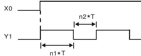
The figure above is common used oscillating circuit for indication light blinks or buzzer alarms. It uses two timers to control On/OFF time of Y1 coil. If figure, n1 and n2 are timer setting of T1 and T2. T is the base of timer (clock period)
