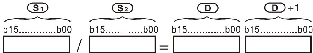
If D is the bit device, it allocates K1~K14 to 16-bit and occupies 2 continuous sets of quotient and remainder.
