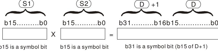
When **D** serves as a bit device, it can designate **K1 ~ K4** and construct a 16-bit result, occupying consecutive 2 groups of 16-bit data.
