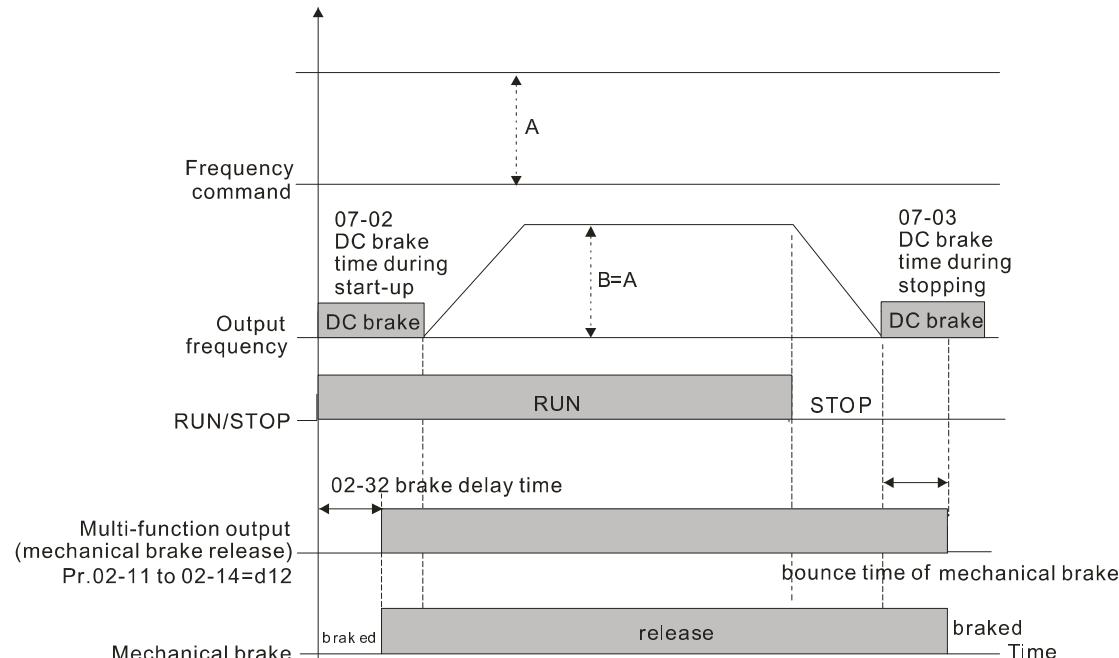
>If this parameter is used without DC brake, it will be invalid. Refer to the following operation timing.
