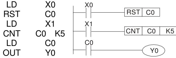
1. When X0=On, RST command is executed, C0 reset to 0 and output contact reset to Off.
