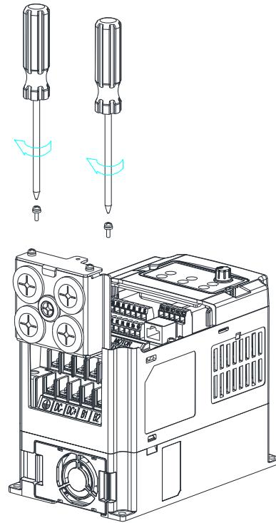
3. Place the wiring cover back and fasten it with screws. Screw M3 torque: 6-8Kg-cm (5.2-6.9lb-in.)
