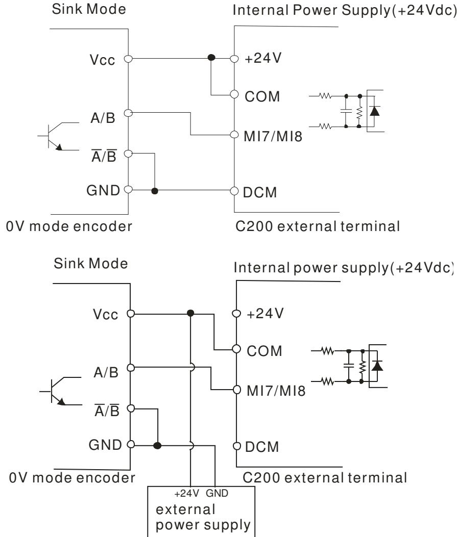
5. Since MI1~MI8 shares the same COM, therefore when using a PG card, MI~MI6 can only be applied at SINK MODE.
