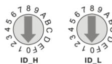
Example: If you need to set up the communication address of CME-COP01 as 26(1AH), simply switch ID\_H to "1" and ID\_L to "A".
