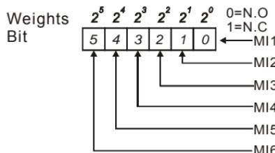
□ The Setting method: It needs to convert binary number (6-bit) to decimal number for input.
