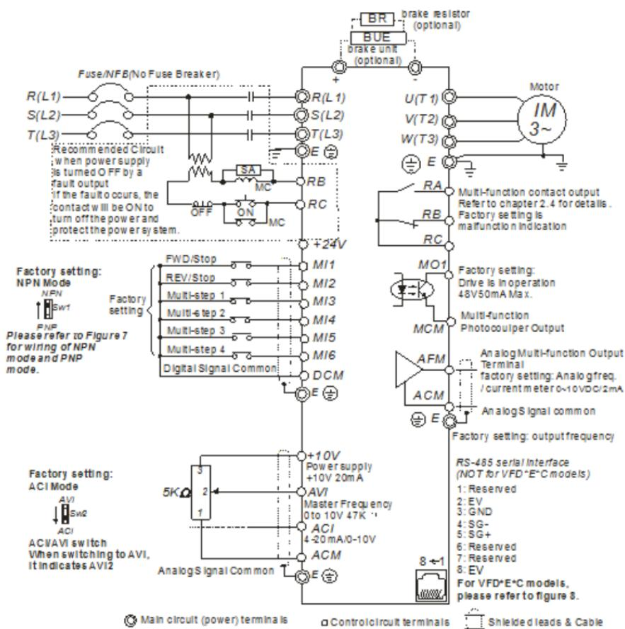
Figure 3 for models of VFD-E Series
