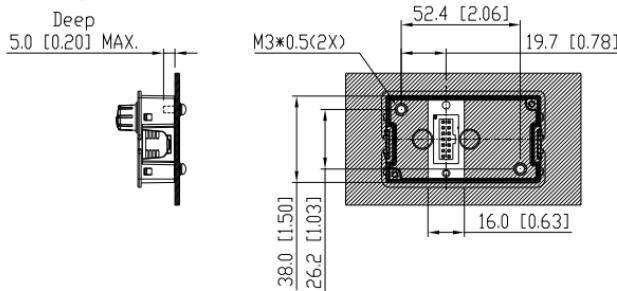
Method2. Install according to plank thickness (Unit: mm [inch])
