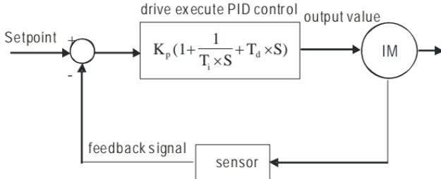
$K_p$ : Proportional gain(P)  $T_i$ : Integral time(I)  $T_d$ : Derivative control(D)  $S$ : Operator
