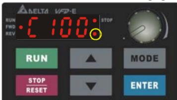
C. 10000~65535 display: It will only display the first 3 digits. The LED at the bottom-right corner and the single decimal point between the middle and the right-most numbers will light to indicate 100 times of the display value. For example, the actual value for the following figure is  $100 \times 100 = 10000$ .
