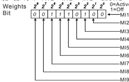
When extension card is installed, the number of the multi-function input terminals will increase according to the extension card. The maximum number of the multi-function input terminals is shown as follows.
