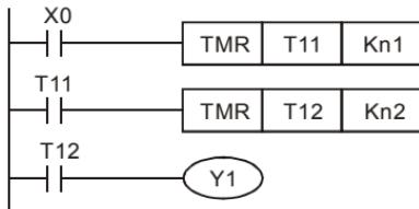
In this circuit, the total delay time from input X0 is close and output Y1 is ON =  $(n1+n2) * T$ . where T is clock period.
