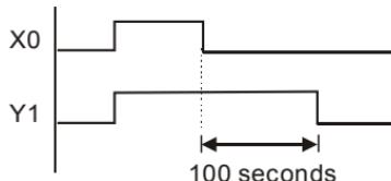
When input X0 is ON, output coil Y1 will be ON at the same time due to the corresponding normally close contact OFF makes timer T10 to be OFF. Output coil Y1 will be OFF after delaying 100 seconds ( $K1000 \times 0.1$  seconds = 100 seconds) once input X0 is OFF and T10 is ON. Please refer to timing chart above.
