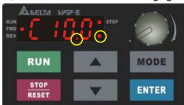
5. When it is changed to "PLC2", RS-485 will be used by PLC.
