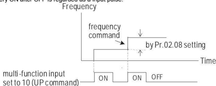
Related parameters: Pr.02.08(Accel/Decel Rate of Change of UP/DOWN Operation with Constant Speed), Pr.04.05(Multi-function Input Terminal (MI3)), Pr.04.06(Multi-function Input Terminal (MI4)), Pr.04.07(Multi-function Input Terminal (MI5)), Pr.04.08(Multi-function Input Terminal (MI6))
