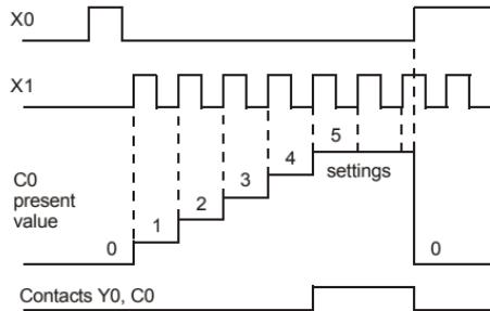
32-bit high-speed addition/subtraction counter C235:
