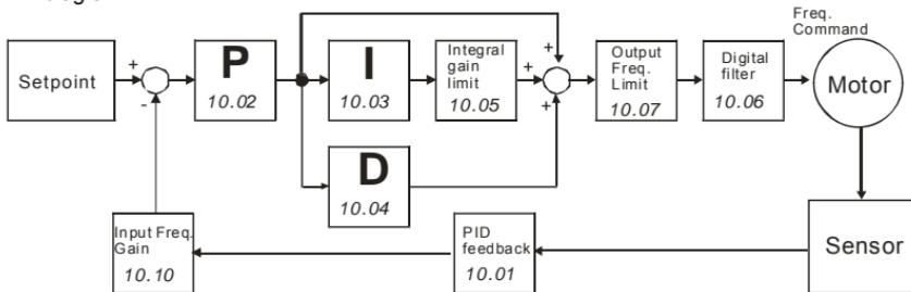
**10.07 PID Output Frequency Limit**
