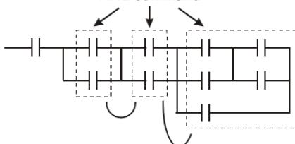
5. ORB command: a block connects to a device or a block in parallel.
