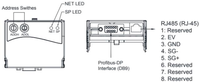
1. SP LED: Indicating the connection status between VFD-E and CME-PD01.
