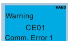
1. Press ENTER and start RESET. If still no response, please contact local distributor or return to the factory. To view the fault DC BUS voltage, output current and output voltage, press "MENU"→"Fault Record".
