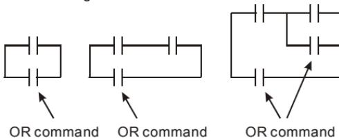
The structures of ORP and ORF are the same but the action is rising-edge or falling-edge.
