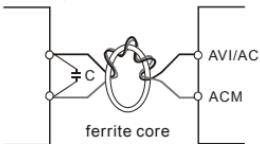
wind each wires 3 times or more around the core
