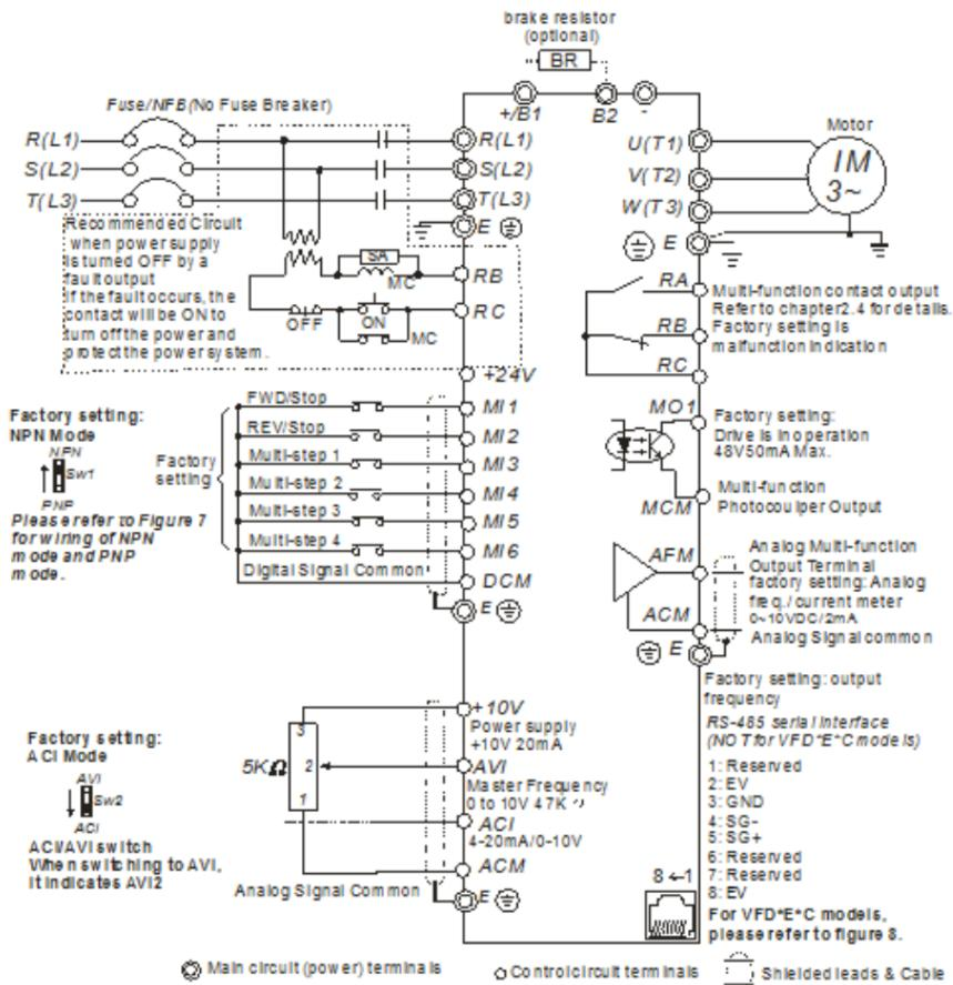
Figure 5 for models of VFD-E Series
