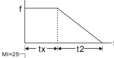
$$S = n \times \left( \frac{t_x + (t_x + t_2)}{2} \right)$$
