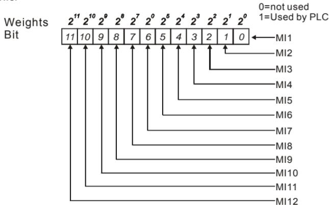
**04.25 The Analog Input Used by PLC (NOT for VFD\*E\*C models)**
