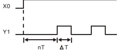
The figure above uses timer T0 to control coil Y1 to be ON. After Y1 is ON, timer T0 will be closed at the next scan period and output Y1. The oscillating circuit will be shown as above. (n is the setting of timer and it is decimal number. T is the base of timer. (clock period))
