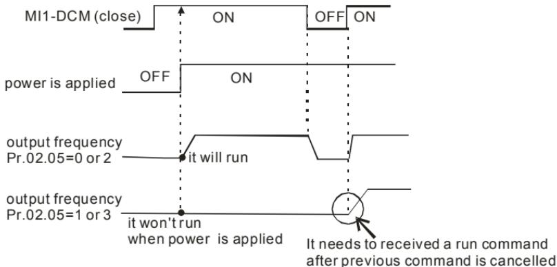
When the operation command source isn't from the external terminals, independently from whether the AC motor drive runs or stops, the AC motor drive will operate according to Pr.02.05 if the two conditions below are both met.
