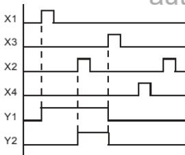
X1 and X3 can start/stop Y1 separately, X2 and X4 can start/stop Y2 separately and they are all self latched circuit. Y1 is an element for Y2 to do AND function due to the normally open contact connects to Y2 in series. Therefore, Y1 is the input of Y2 and Y2 is also the input of Y1.
