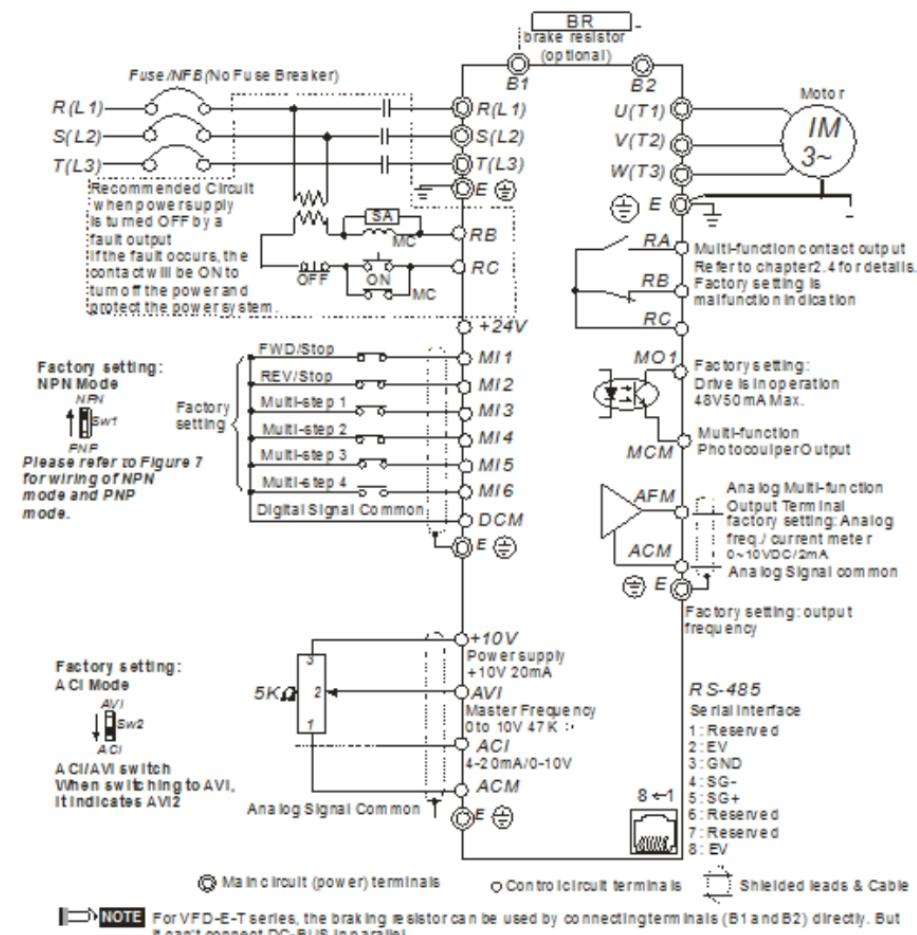
Figure 7 Wiring for NPN mode and PNP mode
