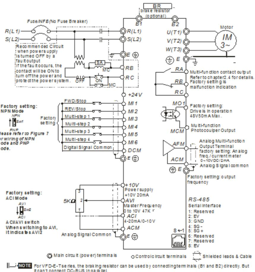
Figure 6 for models of VFD-E Series
