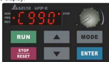
B. 1000 ~ 9999 display: It will only display the first 3 digits. The LED at the bottom-right corner will light to indicate 10 times of the display value. For example, the actual value for the following figure is  $100 \times 10 = 1000$ .
