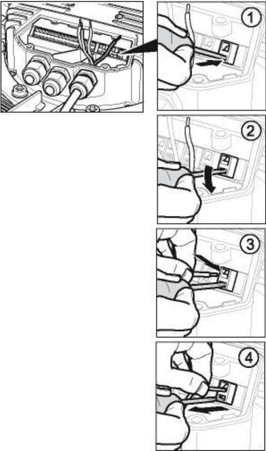
Fig. 2: Connecting wires to terminals
