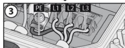
Fig. 3: Connecting wires to terminals
